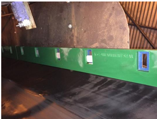
Above and right: K-Containment Seal installed inside the transfer chute.
