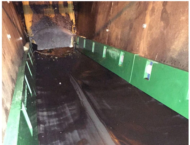
Above and right: K-Containment Seal installed inside the transfer chute.
