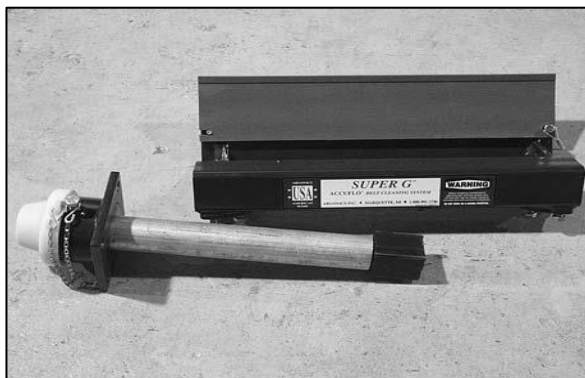
Using a ½" open spanner, loosen the three setscrews located on the bottom of each end of the mainframe. Remove the entire tension cartridge from the left side of the mainframe.
