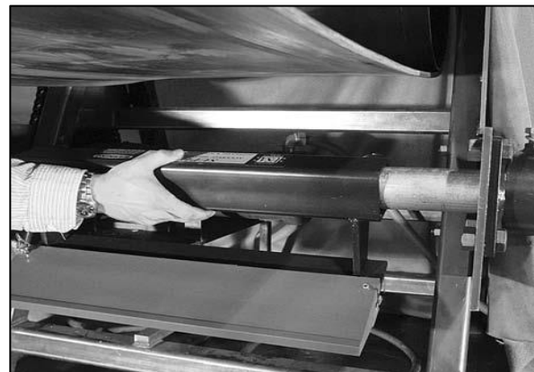
Lift the mainframe into position. Slide the mainframe onto the cartridge, then temporarily retighten the three setscrews on the tensioner side to stabilise system.
