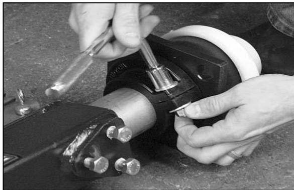
Remove the urethane locking collars from the stub ends.
