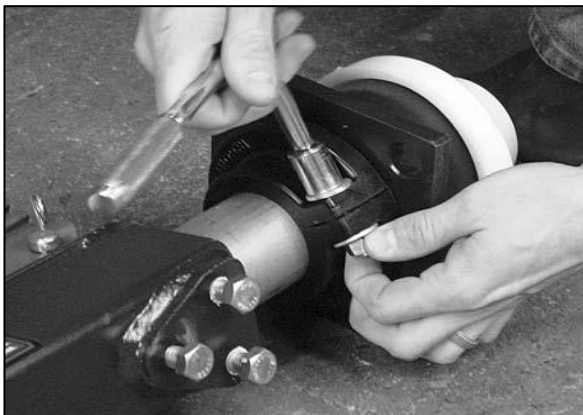
Remove the urethane locking collars from the stub ends.
