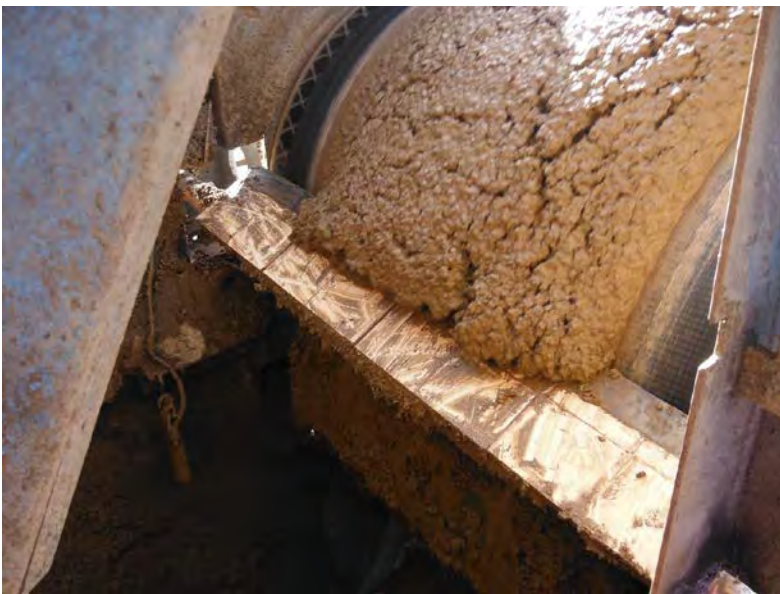
Figure 3: Heavy duty tungsten carbide pre-cleaner in application with cohesive and wet product. (Photo provided by Tecnipak)
