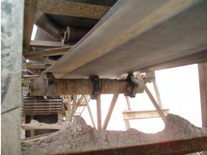
Figure 9 (left): Return roller with retrofit “shaker discs” designed to remove material by vibrating the belt.
