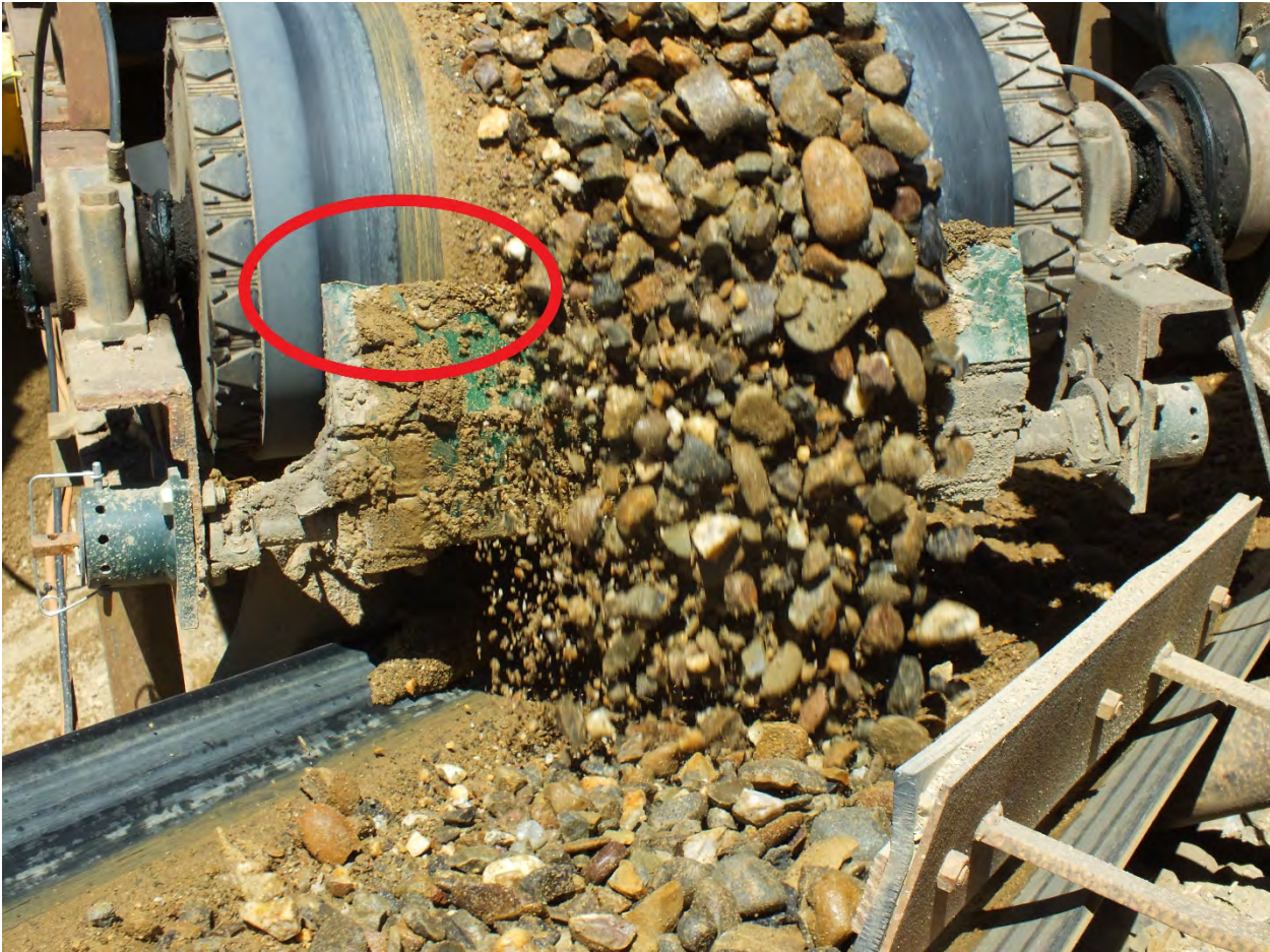
Figure 5: Notice little wear on extreme left edge compared to burden width. This installation would benefit by using a short length blade.
