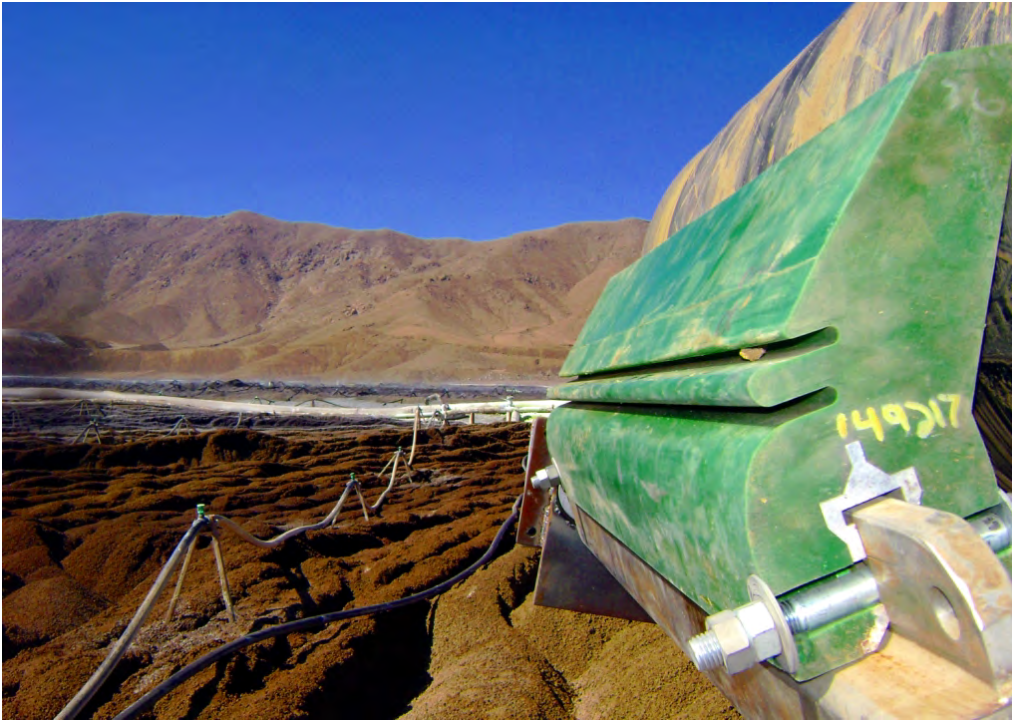
Figure 4: Polyurethane primary cleaner on extremely high capacity belt. (Photo provided by Tecnipak)
