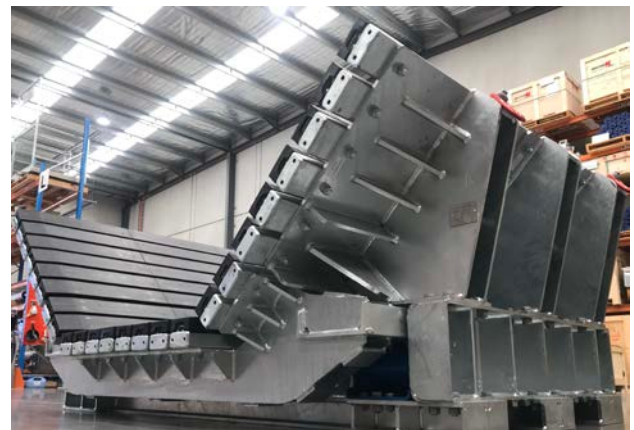
K-Shield Dynamax® Impact Belt Support System XHD Model
