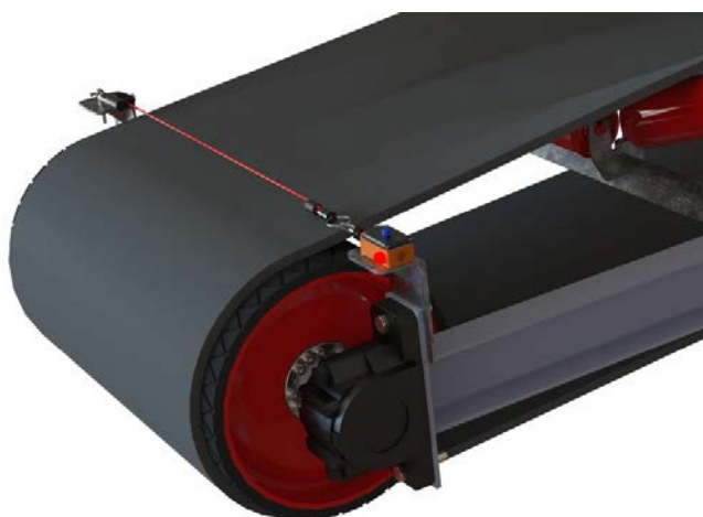
Belt rip detector application across the tail end pulley section.
