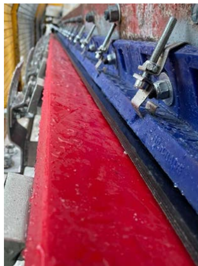
Contactless external skirt and static rail system
